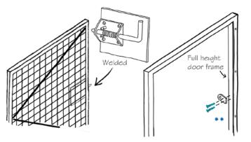
Spring lock is already welded on the door frame and the receiving lock plate
